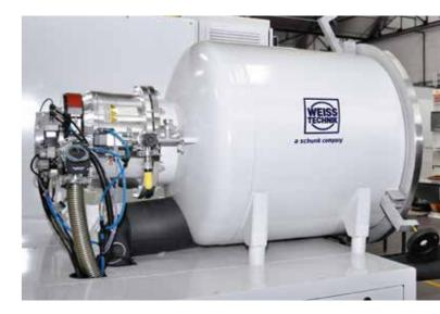
Coolness is regulated through the heat exchanger and the wall plates on the inside of the chamber. The temperature is measured and regulated through sensitive sensors in the vacuum chamber, on the heat exchanger, and on the test object itself. In this way, the vacuum chamber can simulate all temperature and pressure conditions that can exist in space.
