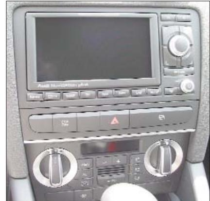
The control and communication system provides the highest level of operating convenience, with the removable, menu-controlled colour touchpanel with graphics-capable display.
