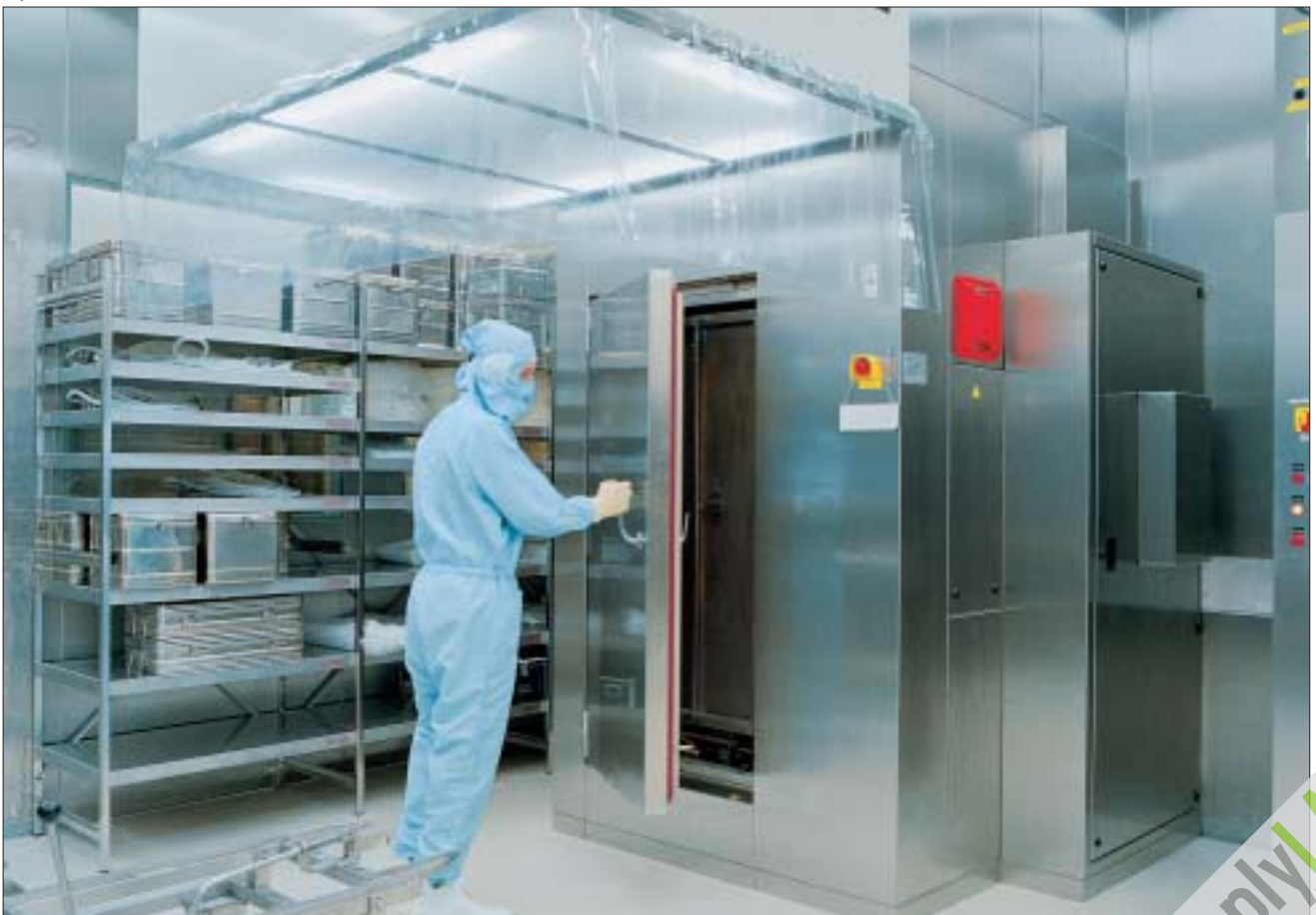
Dry heat steriliser VHSF-K1 with optional cooling chamber (two chamber system) for depyrogenisation
